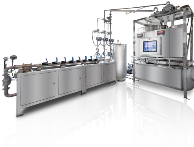
B28 VTB bench is designed for heat meter / water meter calibration and testing procedure. With BOVE's unique design of flow system, weighting system, it supports any ranges of sizing from DN15 to DN600.
